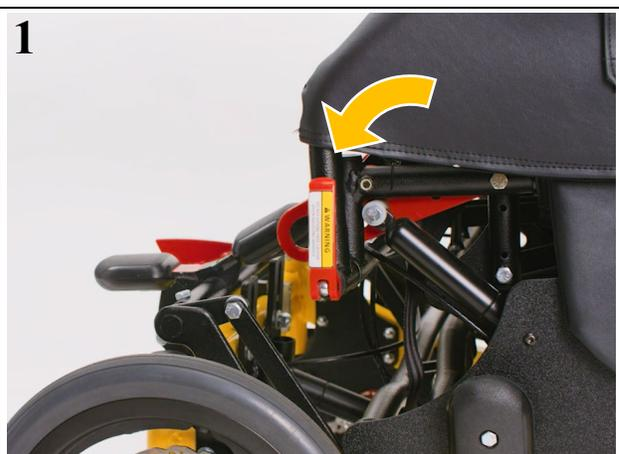
2. If additional width is desired, pull the arms to the desired location, but do not exceed the groove, which is the 2" point.
