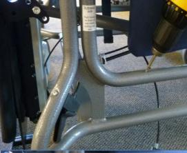
Secure the cable handle to the base frame using the previously drilled hole & self tapping screw.
