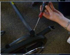
Insert the screw driver into the open tubing, positioning on the rim of the old anti tipper, again using a rubber mallet hammer the end of the screw driver to help loosen and remove. You may need to reposition the screw driver around the rim to loosen all areas before removing.
