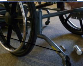
Note: If the existing anti tippers are too difficult to remove, please follow the necessary steps; Remove the black MDLC plug from the top of the caster post, using a flat head screw driver and rubber mallet to hammer the end of the screw driver to pry out the plug, as shown. Try not to damage the plug to allow for re-use.
