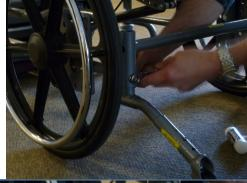
There are three adjustment holes to reach the desired position
