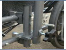
At the top, swaged end, of the IV Pole Holder, insert the IV Pole. Insert the 5/16"- $18 \times 3/8$ " long set screw into one of the weld nuts, at the top of the IV Pole holder. Insert a 5/16"-18 Hand Wheel in the Adjacent Weld Nut.
