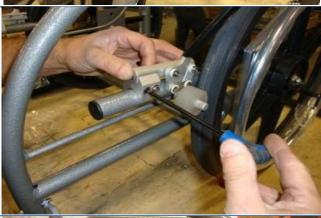
Step 18 - Picture # 2 Continued. (Note: test the wheel lock to ensure the desired amount of force is applied to the tire to put it in a lock position. The closer you mount the aluminum clamp, the tighter the wheel lock will engage)
