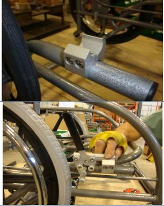
19 Once desired position is achieved, and keeping the wheel lock parallel with side rail of base frame, tighten the screws on the wheel lock clamp using a 5 mm hex key to clamp the lock onto the lock mount.
