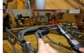
12 Install two 5" total lock casters into the rear legs of the base. Secure casters into the base using 1/4"-20 x 1-1/2" long hex cap screws, 1/4" split lock washers, and 1/4" nylon insert locknuts. Tighten fasteners using 7/16" wrenches. (Heads of the cap screw face the rear of the chair)
