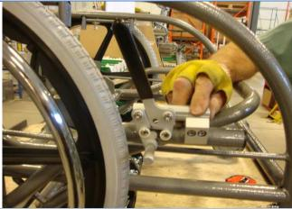
Step 20 - Picture # 2 Continued. (Note: test the wheel lock to ensure the desired amount of force is applied to the tire to put it in a lock position. The closer you mount the aluminum clamp, the tighter the wheel lock will engage)
