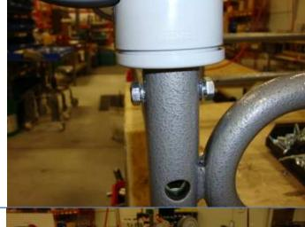
5 Install the 6" directional caster into the caster post with the wheel trailing behind the chair.
