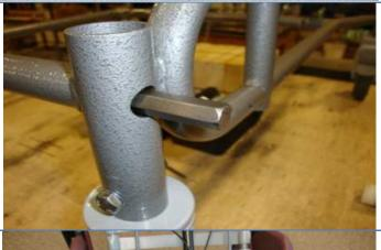
3 Slide the control rod through the non-functioning caster far enough to allow the caster to be removed from the base frame. Ensure the functioning caster is in and remains in directional mode until the replacement is complete.
