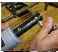
Install the Hex Rod through the hole located in the outside wall of the caster post through the casters, leaving approx. the same amount exposed on both sides.
