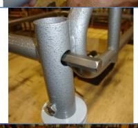
Install the left and right MDLC Pedals onto the left and right side of the base respectively. Tighten with the 5/32" Allen wrench. Insure that the MDLC pedals are set to the directional mode upon installation. See the corresponding image.
