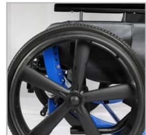
*Quick-release mag wheels can be removed for easy storage*
