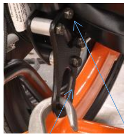
Rear Securement with wheelchair anchored seat belt anchor
